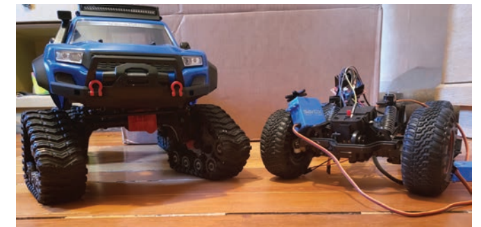
Built by ECE students Sherman White and Jina Yoo, the team’s first prototype (right) and more recent prototype (left), which features a track mounted design for better traction in wet soil.
